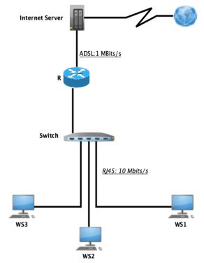
We want to transfer a 3 KBytes file from station WS1 to the Router R :
